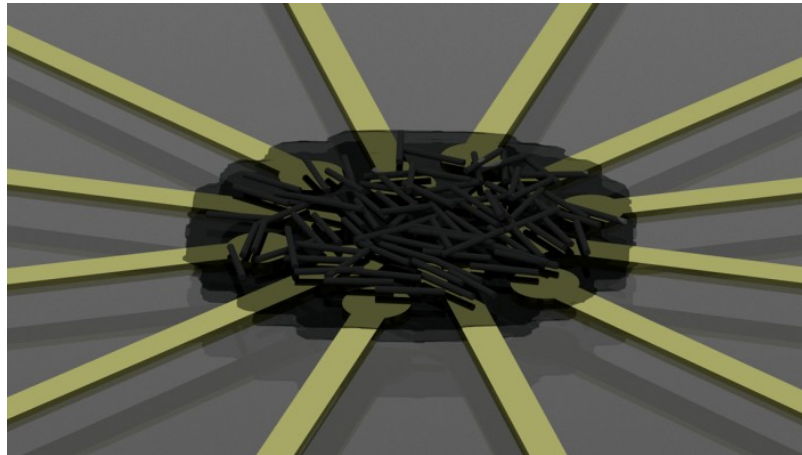
Carbon nanotubes deposited on a microelectrode array. EU project NASCENCE (2015)
