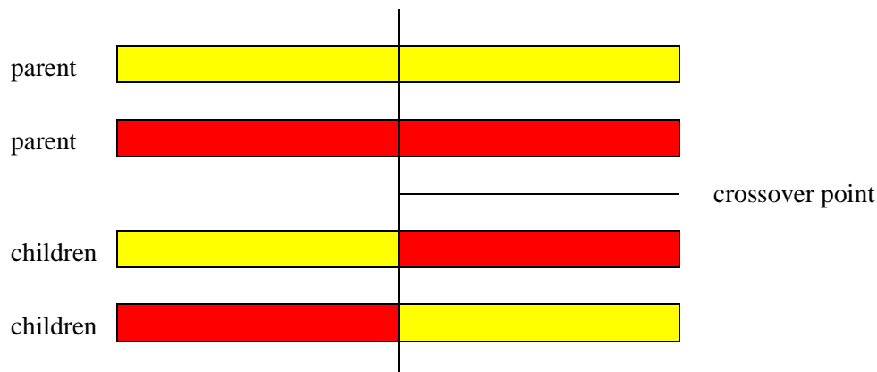
FIGURE 4: One-point uniform crossover: a single crossover point on both parents' organism strings is selected. All data beyond that point in either organism string is swapped between the two parent organisms. The resulting organisms are the children.
